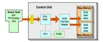
Figure 3. Airborne data flow and recording for ADS
