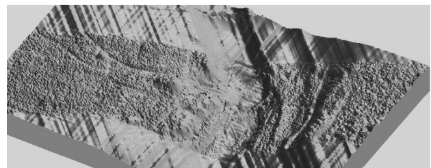
Figure 5 DHM – filtered (with break lines)
