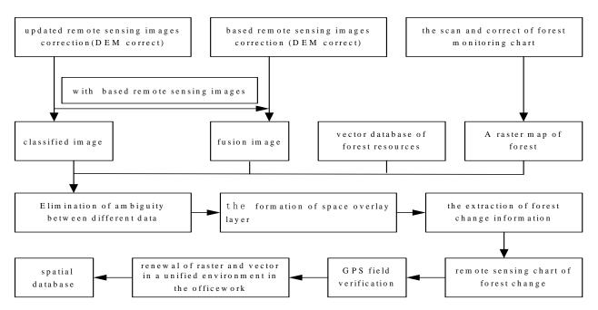
Figure 2. The Flow Chart of the Integration Renewal of Vector and Grid Forest Monitoring Map Based on 3S Technology
