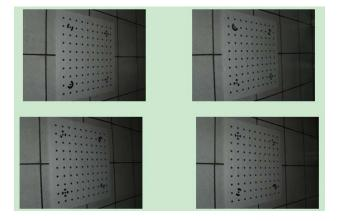
Fig.2 The second four images of the model plane. They are photographed with the camera rotated 90 degrees anticlockwise.
