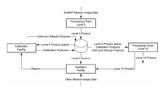
Figure 1. Calibration, Validation, and Processing Chain
