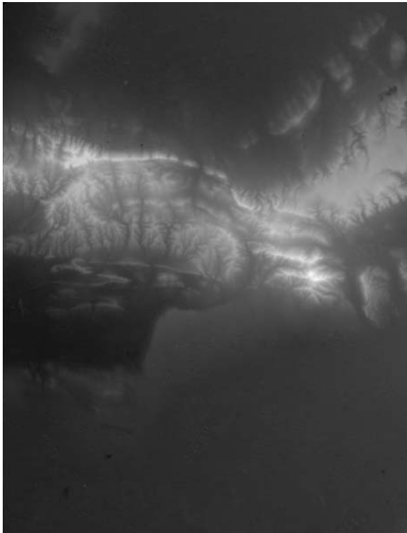
Figure 3: DSM in overlap area of stereo pairs M1/2 (grid spacing 10 m, size of area 17.9 km x 23.5 km)
