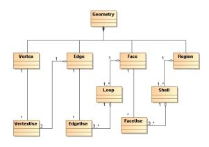
Figure 1. 3D spatial data model based on the principle of cell complex
