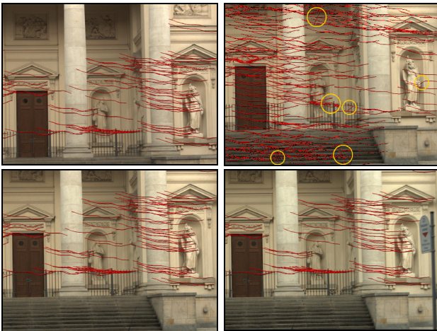
Figure 9. Image triplet overlaid with permanent tracked features over 10 frames compared to the KLT (top right)
