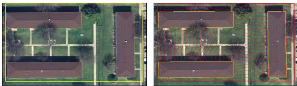
Figure 4. Boundary extraction of multiple buildings [upper: Initial boundary (yellow), lower: boundary evolution (red) and extracted boundaries (yellow)]
