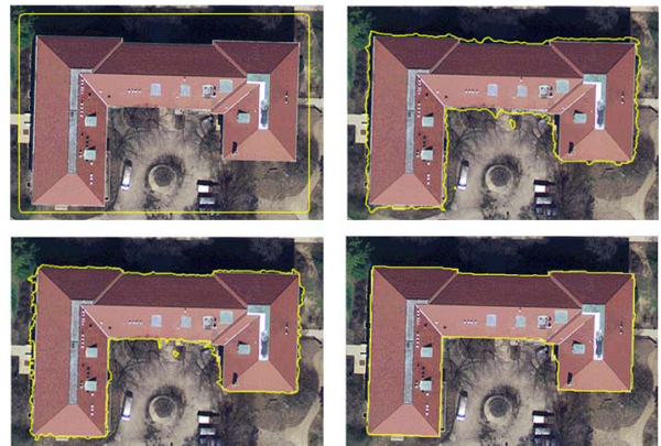
Figure 3. Building boundary extraction using active contour (upper: Initial boundary, boundary evolution result with 21x21 window; lower; result with 11x11 window, result with 3x3 window as final building extraction)
