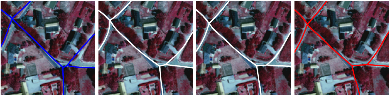
Figure 4. Refinement of a road network in a suburban area with network snakes including the topology-preserving energy: initialization (blue), optimization steps (white) and result (red)
