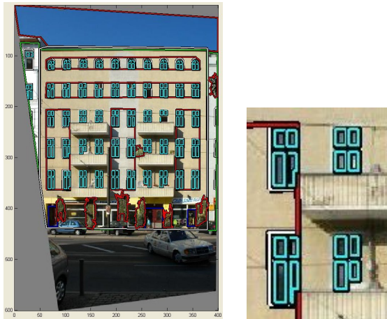
Figure 1: Rectified facade image and an detail from eTRIMS data base with manually annotated regions, e. g. window panes, vegetation.
