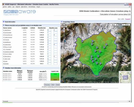
Figure 4. Calculation and visualization of the elevation zones of a watershed.
