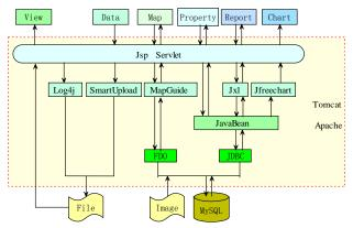
Figure 2. Graph showing the architecture design of the system
