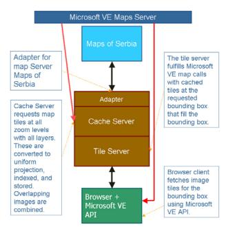
Figure 8. Architecture of application based on Microsoft VE, MapSoft Tile and Cache server
