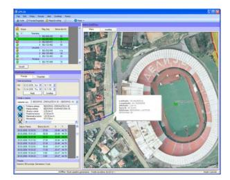
Figure 9. Application for automatic vehicle location (AVL) where MapsOfSerbia and Microsoft VE are integrated
