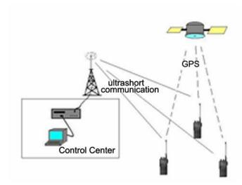
Figure 2. Hardware configuration for forest fire control commanding and decision making system
