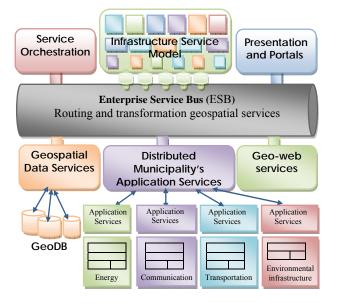
Figure 1. Component of enterprise service bus
