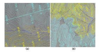
Figure 6. Automated mosaic of cartographic maps. (A is the stereoscopic view in a workstation and B is the stereoscopic view of the same ground area in another workstation. Yellow contours are measured in location workstation. The blues are measured in another workstation)
