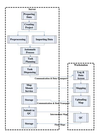
Figure 7. Workflows of seamless mapping system
