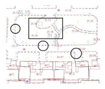
Figure 3 Differences between 1:500 and 1:1000 DLG
