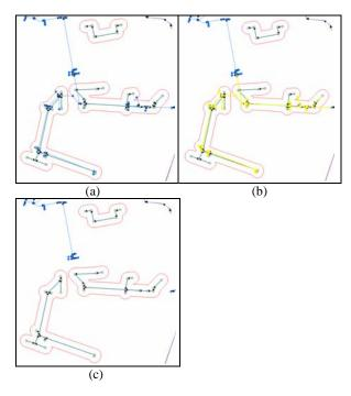
Figure 13. The Process of Updating Existing Database.(a) Create a 10 m Buffer,(b) Selecting the Existing Data in the Buffer,(c) The Result after Deleting the Selected Dataset.
