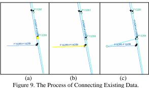
(a) Zoom in the Area for Selecting LOST;(b) Highlight the Existing Pipe;(c) The Connecting Result
