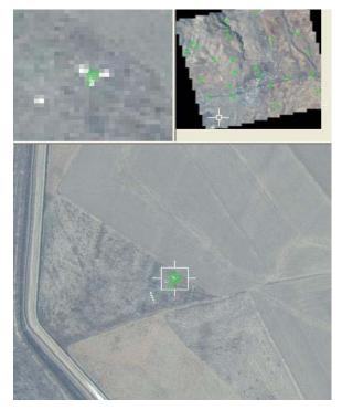
Figure 3. A GCP marked on the ground.
