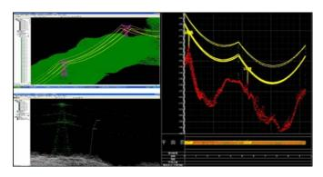
Figure 8. dangerous points checking
