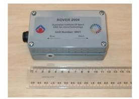
Figure 7. A compact prototype rower monitoring and coaching system (ROVER-2004) with 10 Hz carrier GPS capability and wireless communication.
