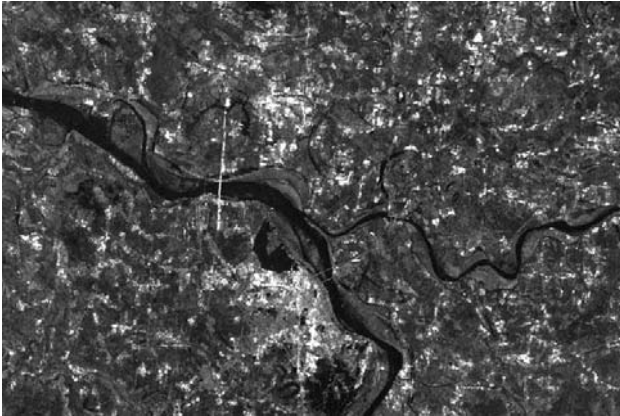
Figure 1. JERS1-SAR image 30m resolution after GAMMA 3X3 FILTER and Orthogonal Geometric Correction
