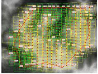
Figure 5: Planning over DTM causes interesting footprints as presented with an example with high relief
