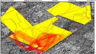
Figure 11: Typical track of the helicopter used for forest chalking. Without a FMS a homogeneous coverage is nearly impossible
