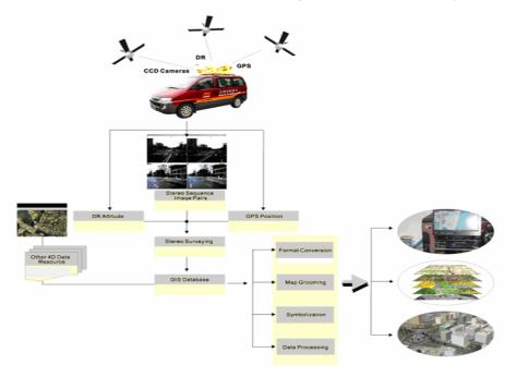
Figure 6. The working principle of VisionCruiserTM
