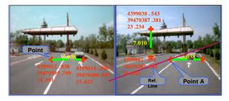
Figure 13. Measurement of road width and object height by end users on web
