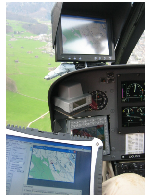
Figure 7: Standard setup of HELIPOS in the cockpit: Controller view (bottom screen), pilot view as an extended screen on 8inch - monitor (top)
