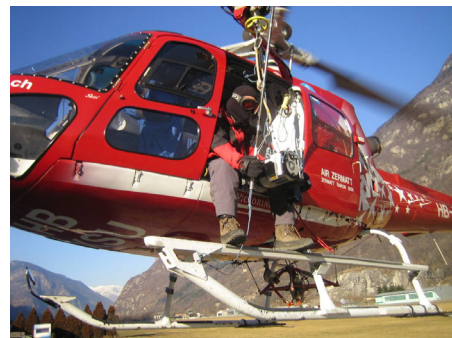
Figure 2: Handheld mapping system (Scan2map) installed in a helicopter
