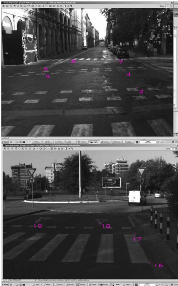
Figure 6. Example of ground point used for the comparison with GPS/RTK survey identified on the images acquired by the Road-Scanner system
