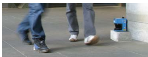
Figure 1. Sensor alignment scanning pedestrians' feet
