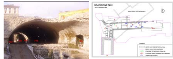
Figure 2. Laser scanner positioning
