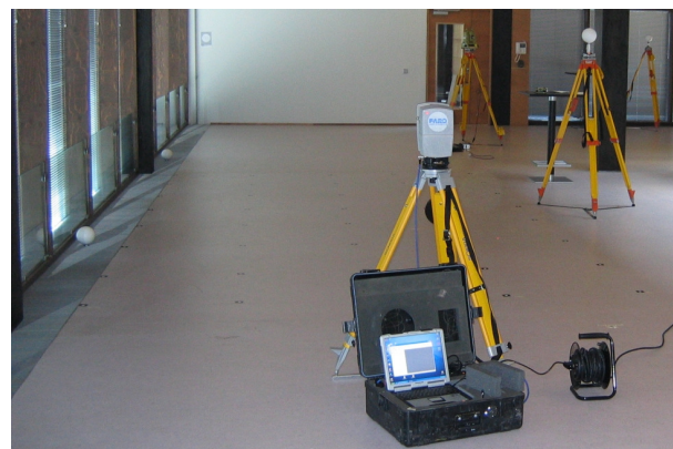
Figure 3. Laser scanning of the floor. Laser scanner on tripod in front of the image (station 6), photogrammetric targets on the floor behind the scanner, spherical reference targets on the floor (left) and on tripods (right) and one paper reference target on the wall (upper left).
