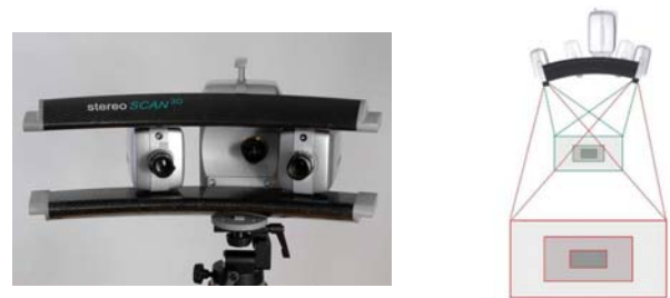
Figure 7a and 7b. Breuckmann StereoSCAN 3D and Camera Setup
