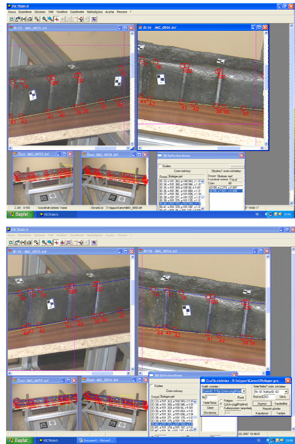
Figure 4. Photogrammetric evaluation steps at PICTRAN
