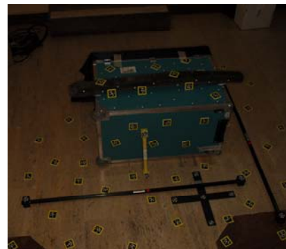
Figure 8. Determination of indeks marks coordinates by photogrammetric method
