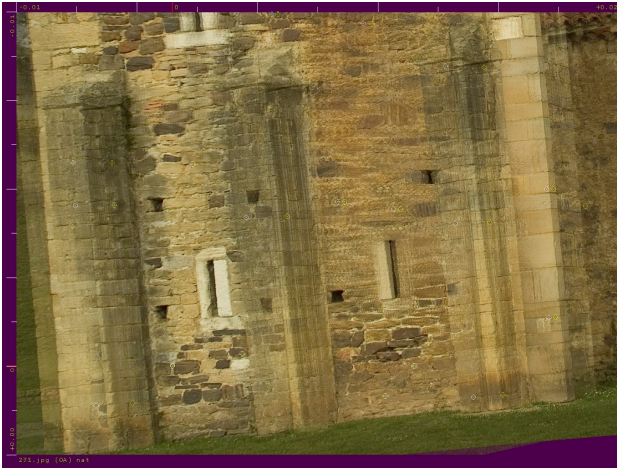
Figure 2. Two projections overlapped on the same single plane. Left window is closer to approximate plane, so looks sharper
