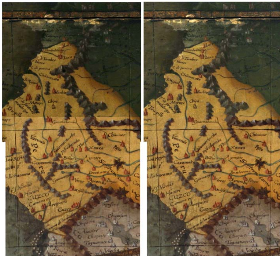
Figure 8. Left: A stitched mosaic of parts of three rectified images of a slice of the sphere. In the upper part a clear seamline is visible. Right: The radiometrically corrected image.
