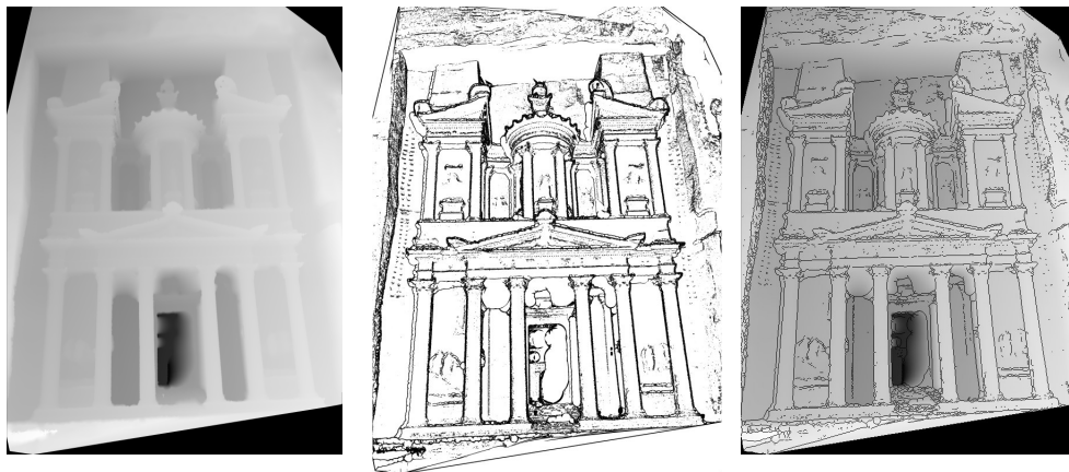
Figure 7. a) Range images collected from Petra treasury (Al-Khasneh). b) Segmentation results using mask size 11. c) Edge map projected in the range image after skeletonized.
