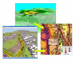
Figure 7: generation of noise pollution maps by noise dispersion simulation; result visualization using web services
