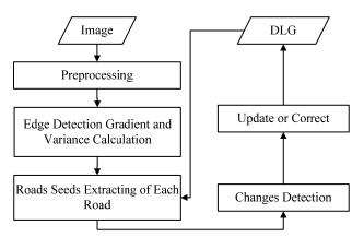
Figure 5: The Whole Work Flow for Roads Changes Detection
