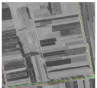
Figure 7: Part of The Original Image, The Poor GIS Data and The Extracted Road Line
