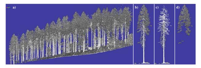
Figure 1. Example of the merged LiDAR scans of the open forest edge at the first scanning location (a). Example of one individual tree (b), separated wood (c) and leaf (d) biomass.
