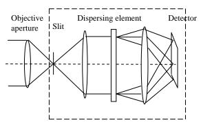
Figure 2: The optical head model of a hyperspectral imager
