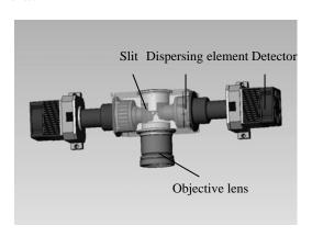
Figure 5: the optical head of wide field of view hyperspectral imager
