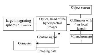
Figure 7: layout of calibration of the wide field of view hyperspectral imager
