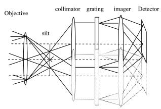
Figure 4: The optical head model of wide field of view hyperspectral imager that the field of view of hyperspectral imager is widen.
