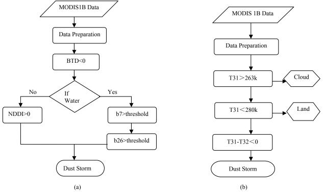
Figure 3. The concrete process for dust storm detection :(a) at daytime ;(b)at nighttime.
