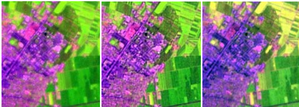
Figure1.HPF fused image 543 bands Figure2.SFIM fused image 543bands Figure3. Brovery fused image 543bands
