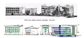
Figure 6. Detailed map of building façades using laser scanning data - laser scanning data (top) and façade plan (bottom)
