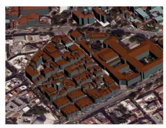
Figure 10. 3D city model of Istanbul Historic Peninsula as LoD2 in the Suleymaniye area superimposed on an orthophoto as an overview (top) and detailed view (bottom)
