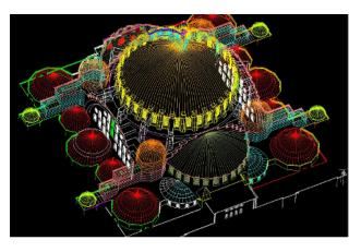
Figure 14. Wireframe of the Suleymaniye Mosque 3D model
