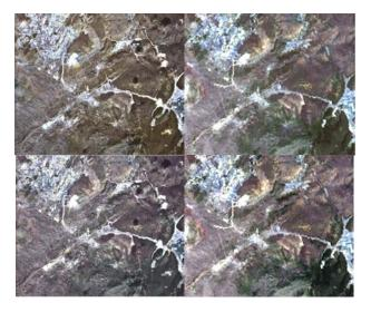
Figure 6. Merged imageries (a: Brovey Transform, b: IHS, c: Principal Component, d: Resampled Landsat multispectral)
