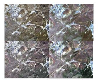
Figure 2. Merged imageries (a: Brovey Transform, b: IHS, c: Principal Component, d: Landsat multispectral)
