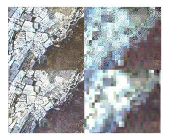
Figure 3. Merged imageries (a: Brovey Transform, b: IHS, c: Principal Component, d: Landsat multispectral)
