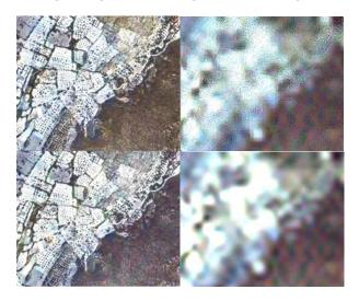
Figure 7. Merged imageries (a: Brovey Transform, b: IHS, c: Principal Component, d: Resampled Landsat multispectral)
