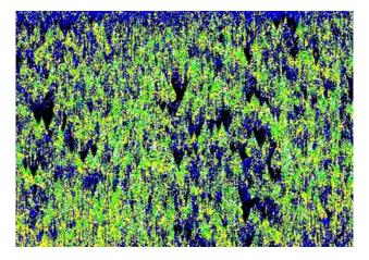
Figure 4. Backscatter phase centre height derived from simulated InSAR L-band HH images of a 150m by 200m stem map in Howland, Maine. Mean height is 5.07m with a standard deviation of 10.8m. Blue : 0-5m, Yellow: 5-10m Green:10-15m white:>15m.
