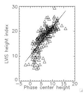
Figure 7. The correlation between 100% energy height (H100) and the phase centre height.
