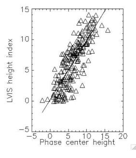
Figure 6. The correlation between 50% energy height (H50) and the phase centre height.
