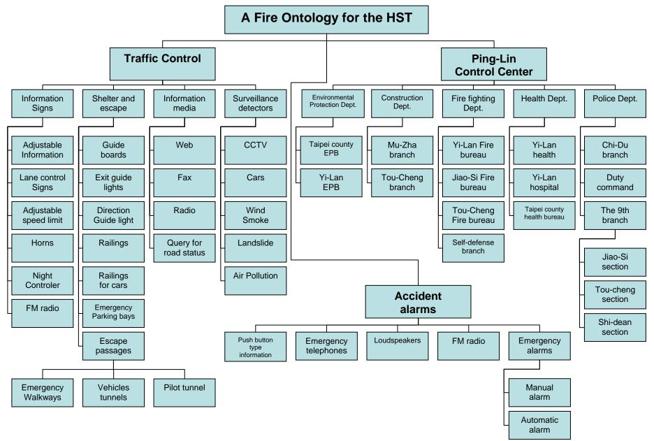
Figure 4. An Ontology for safety features of the Hsueh-Shan Tunnel (HST) (1/2)
