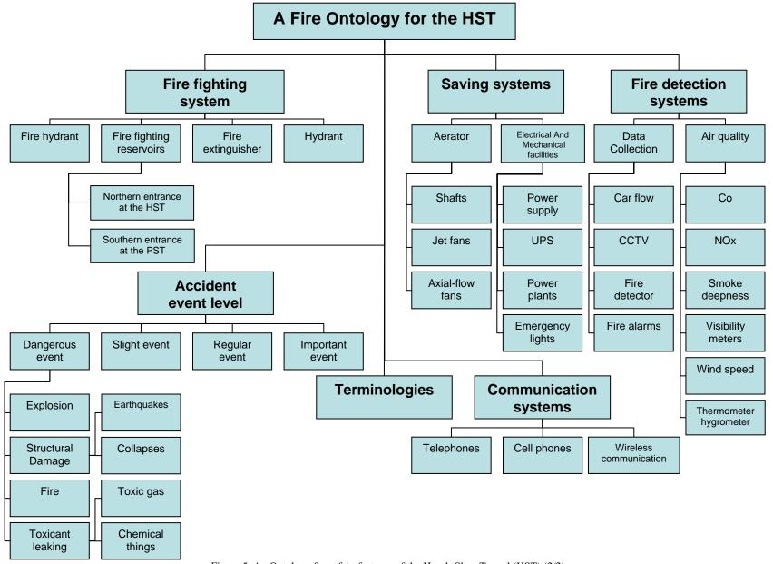
Figure 5. An Ontology for safety features of the Hsueh-Shan Tunnel (HST) (2/2)
