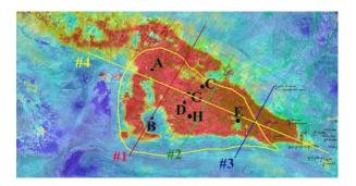
Figure 6. Hypothetical confined aquifer system boundary superimposed on the averaged interferogram.
