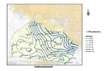
Figure 4. Water table decline contours and the locations of piezometers
