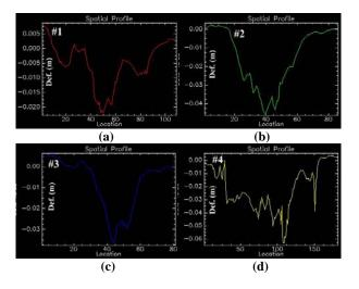
Figure 3. Constructed Profiles using interferogram 1. (a) profile #1, (b) profile #2, (c) profile #3 and (d) profile #4
