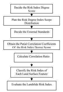
Figure.3 The technical flow-chart of landslide risk index estimation based on Quantification Theory II Analysis
