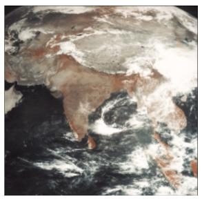
Image acquired by the Indian INSAT-2E which was launched at 2 April 1999. The CCD camera records in the visible, near and medium infrared wavelengths at 1 km ground resolution. Its orbit and swath enable a potential revisit time of 30 minutes within its total field of view and makes it suitable for disaster monitoring.
