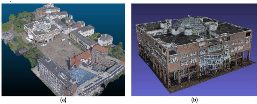
Figure 4: Example of dense point clouds generated from airborne oblique images (a) and co-registered UAV and terrestrial images, both showing the city hall (and square, in (a)).
