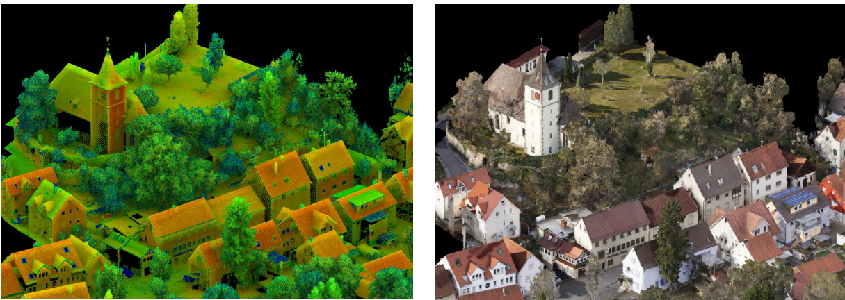
Figure 2: Subset of our proposed benchmark datasets. The high-resolution LiDAR data H3D(PC) ( left; coloured according to reflectance ) is manually annotated and labels are transferred to the 3D textured mesh H3D (Mesh) ( right ).
