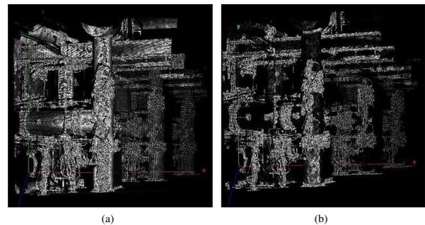
Figure 1. (a) Gray scale image of the curvature index vs (b) variance of curvature index applied to an industrial scene. Notice contrast between curvature and variance of curvature for the pipes
