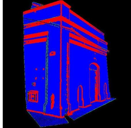
Figure 2. Point cloud from a section of the Midland rail yards in Perth, Western Australia. The classification results are shown with blue representing surfaces, red representing edges and green representing boundaries.
