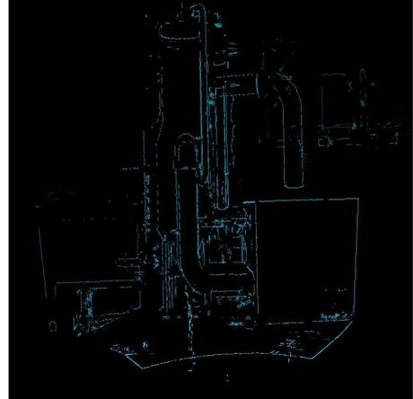
Figure 9. The local intersection applied to the cyclone test data set as well as the boundary points to define the extents of the segmented surfaces.
