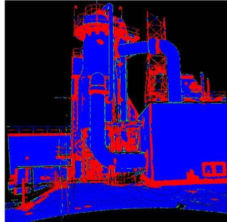
Figure 3. Leica test data of an industrial plant. The classification results are shown with blue representing surfaces, red representing edges and green representing boundaries.
