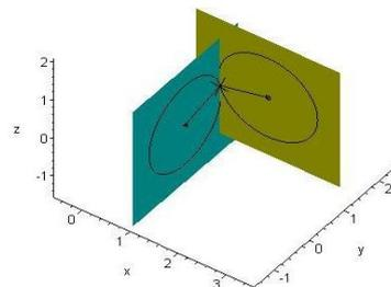
Figure 7. The local intersection point of two surface points defined by where the circles met
